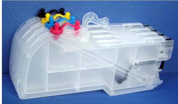
**Items needed: gloves, Black Dye, Cyan, Magenta, Yellow inks, paper towels, review hints & tips and check list. Note: Plug fill-hole with plug that comes with the empty refillable cartridges. Unplug air vent hole plug after refilling and before you use in printer. Large hole and large plug are your fill hole. Small plug and your small plug is your air vent hole.**
