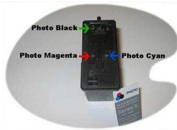
**Items needed: gloves, hand-drill, #6 refill station, Syringe , needle tip, Use Black Dye for Photo Black Photo cyan and Photo magenta , paper towels, review hints & tips and check list Note: Do not use the refill station lid for refilling this cartridge. Do not plug fill-hole after filling**
