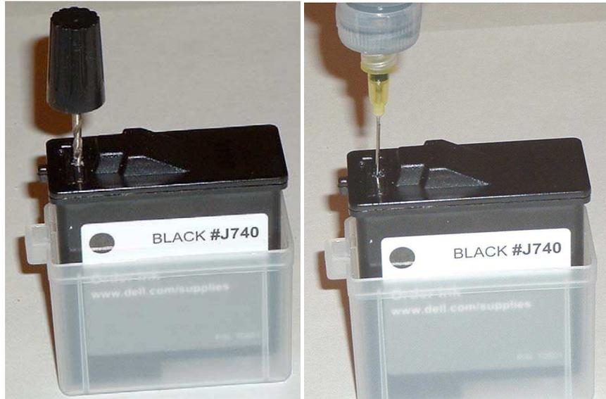
**Items Needed: gloves, #6 refill station, hand-drill, dye-based ink, paper towels, review hints & tips and check list Note: Do not use the refill station lid for refilling this cartridge.**
