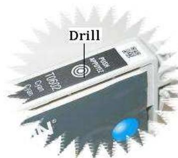
1) Put the cartridge on some paper towels in an area where you can tolerate a spill. You may wish to wear the rubber gloves provided if you don't wish to temporarily stain your fingers. Place the cartridge so that the ink exit hole is pointing down and is on the surface in front of you. The Epson Label should be pointing towards your chest. This is the Front side of the cartridge.
